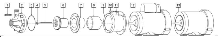
NOTE: The Impeller, shaft, and Thrust washer are packed separately within the carton to prevent damage during shipping. These items need to be assembled into the pump before installation. Be sure all parts are assembled per the exploded view shown.
