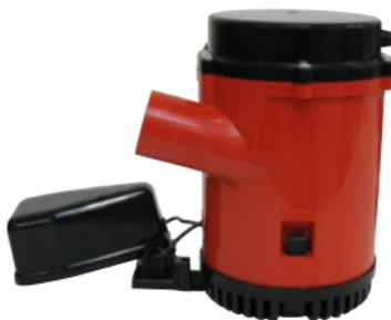
equipped with a T-mount. AS888 should always be installed in parallel to the keel with the floating body directed aft. Never install AS888 at a level lower than the inlet of the bilge pump.
