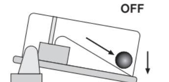
Ball at rest, switch in off mode.
