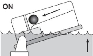
Water raises switch, ball rolls back, switch snaps on.
